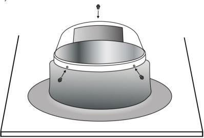
Fit the dome protection ring down over the dome, with the holes within the ring locating onto the dome spacers as shown below.
