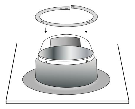
Drive the roof dome screws through the dome spacers to fix both the roof dome and protection ring into place. The screws should pierce through both the roof flashing and the inside of the reflective tube. Do not overtighten the screws or you may cause damage to the roof dome.
