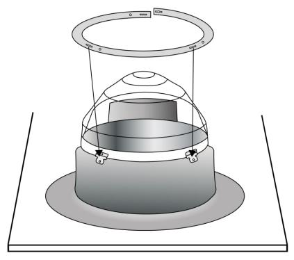
Bend the fixing tabs upwards to fix the protection ring into place.
