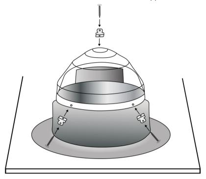
Fit the dome protection ring down over the dome, with the slots within the ring locating onto the fixing tabs as shown below.
